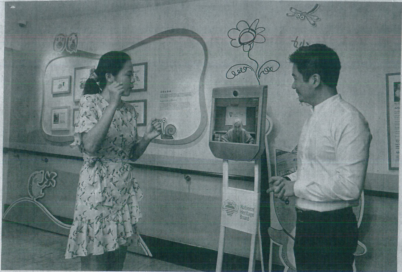
Mr Alvin Tan, assistant chief executive of the National Heritage Board, and Ms Lu Cai Xia, assistant curator of the Sun Yat Sen Nanyang Memorial Hall, with the remote-controlled Telepresence Robot. With the robot, a visitor needs only a device with a video camera and microphone, like a laptop or smartphone, as well as Wi-Fi to take a virtual tour. ST PHOTO: GIN TAY
